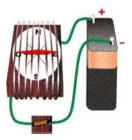
Öersted discovered that electric currents produce magnetic fields with lines of force that form concentric circles around the current. Magnetic fields are created by particles in movement.
